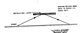
Fig. 14 Refraction of Radar Beam
