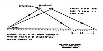
Fig. 12 Profile View Showing Effect of Moving Reflector
