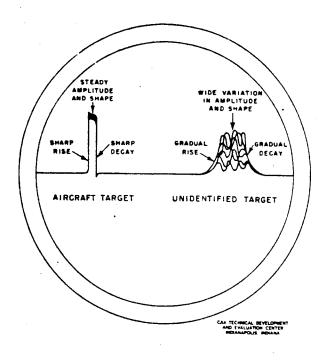
Fig. 15 Comparative A-Scope Target Displays
