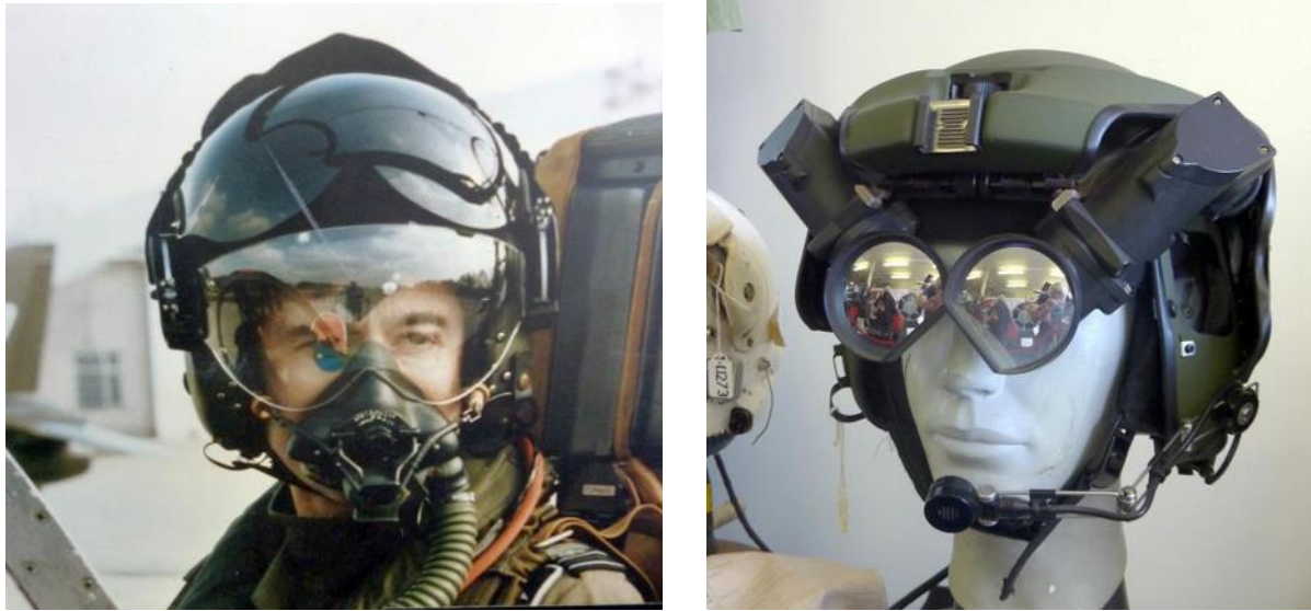
Figure 34. An experimental helmet mounted sight (left) which completed laboratory, simulator and extensive flight trials in RAEs Jaguar aircraft before going into production and operational use for Jaguar, Harrier and Tornado. The experimental binocular helmet mounted display (HMD) on the right was tested in flight in Lynx and in the Bedford helicopter simulator
