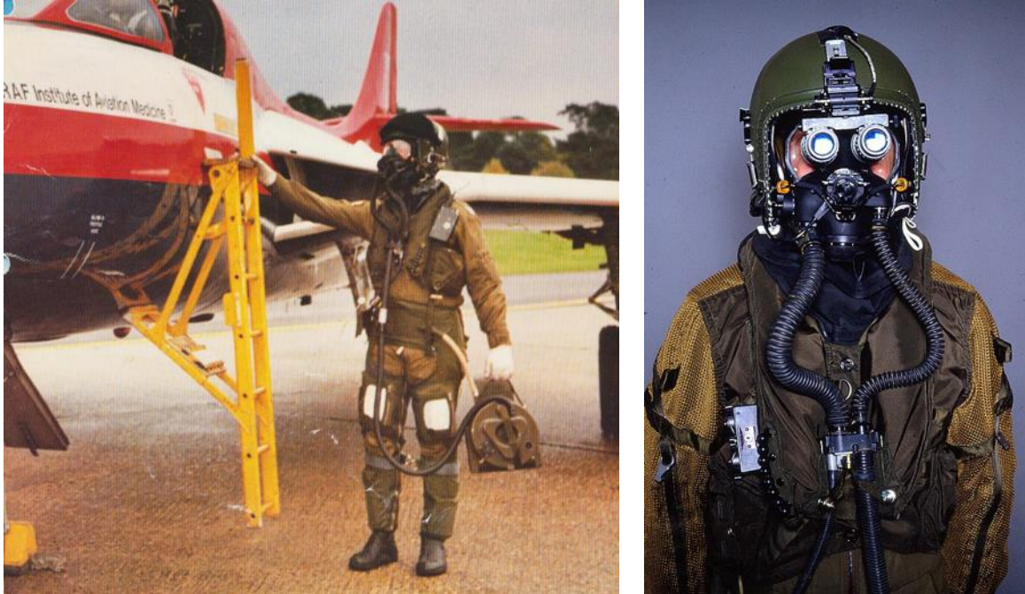
Figure 25. Flight testing of the AR5 NBC Respirator was carried out in the RAF IAM Hunter shown here with the pilot holding its ground ventilator (the 'Whistling Handbag'). The AR5 on the right is worn with Night Vision Goggles
