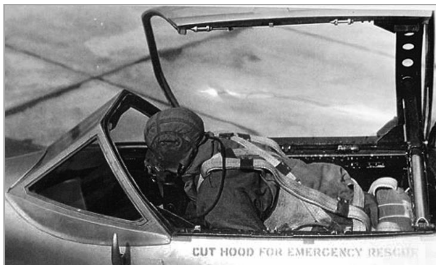
Figure 40 The prone piloting position in the experimental Meteor
