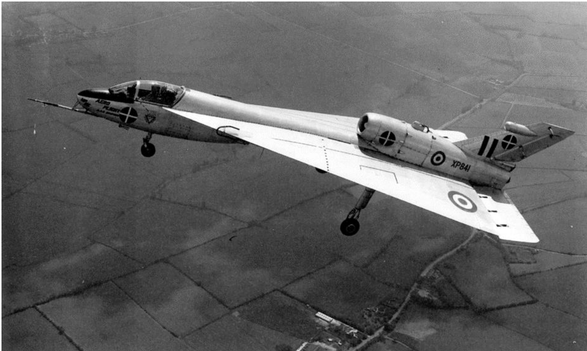
Figure 29. The simple Handley Page HP.115 was built and flown to confirm the basic design and wind-tunnel tests of the aerodynamics of the proposed high-angle approach to landing for Concorde. Over 1000 flights from RAE Bedford were performed with this unique aircraft.
