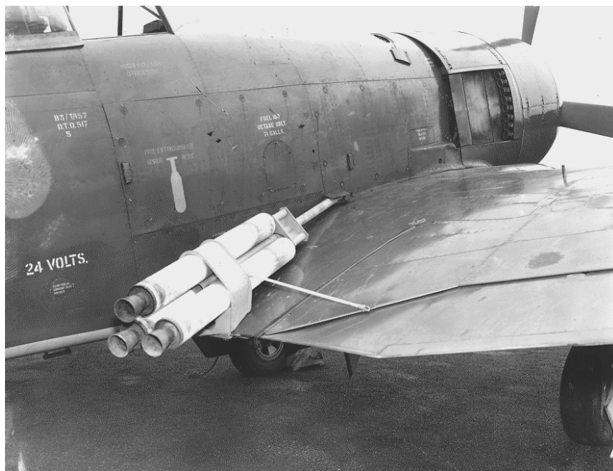
Figure 22. The trials installation in June 1946 of a rocket pack on one side of a Blackburn Firebrand III prior to rocket assisted take-off (RATO) experiments using three 5 inch cordite rockets on either side.
