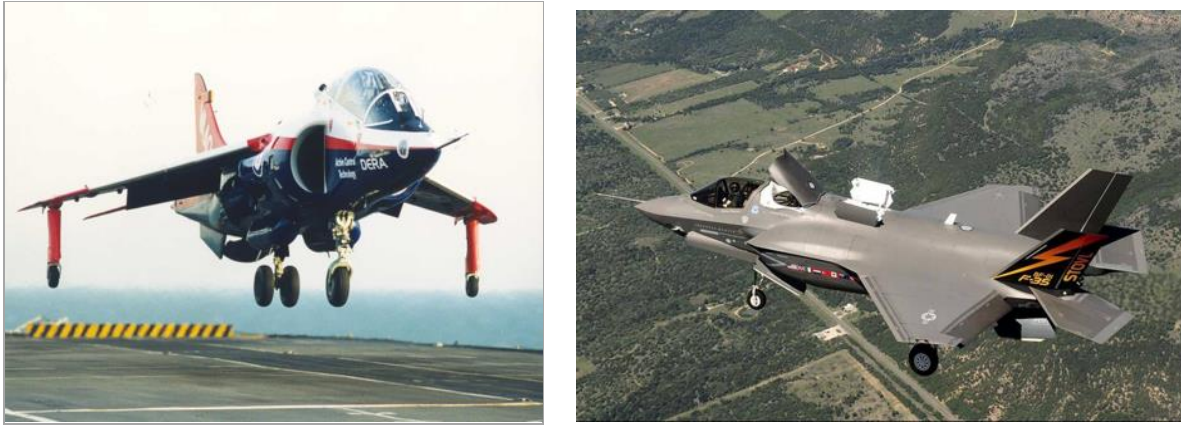
Figure 35. In 2002 the Bedford Unified Control concept was selected for the JSF STOVL variant. The VAAC Harrier (left) and JSF BF-01 (right) hovering under the flight control of the Unified Control method
