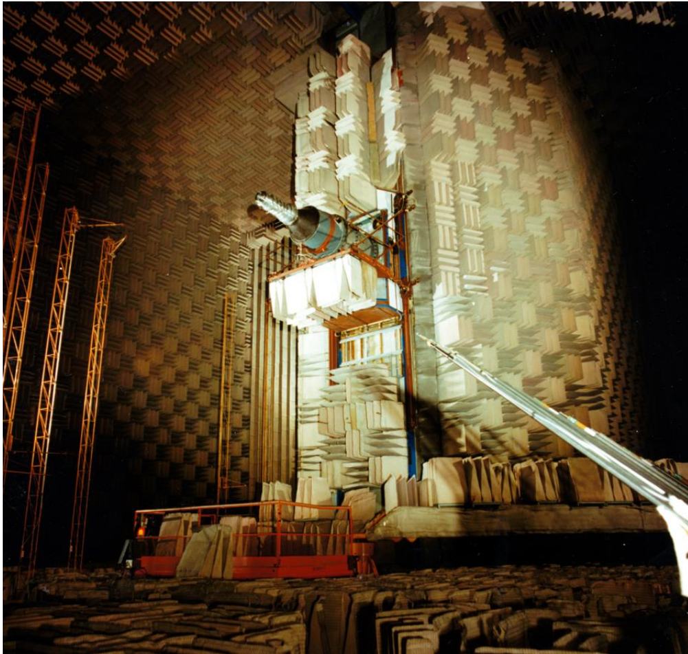
Figure 19. The anechoic facility comprised an acoustically lined main test chamber 85ft wide and 46ft high with an overall length of 88ft, of which 52ft formed the working section. The jet flow from the main noise source was projected towards an acoustically lined, flared duct 28ft diameter at inlet with a 20ft diameter throat, which acted as an exhaust inducer.
