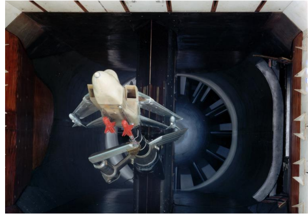
Figure 10. The Transonic tunnel facilities were developed such that any aerodynamic interferences during weapon release at high-speed could be studied prior to flight trials
