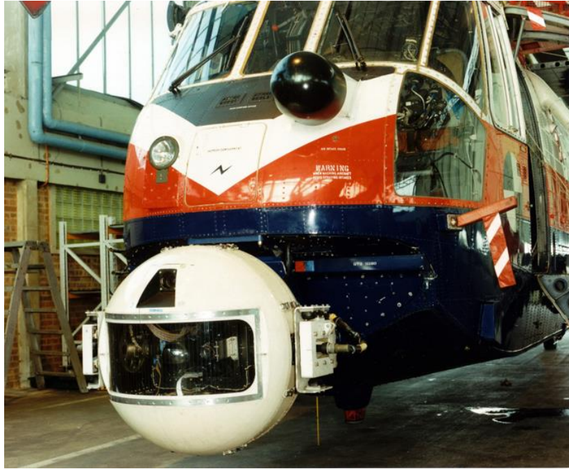
Figure 26. Early helicopter trials with enhanced vision devices led to further developments, as technologies improved and advanced, in later Sea Kings and Pumas as part of the RAE day / night all-weather (DNAW) research programmes. Other programmes covering all aspects of helicopter technology and operational use were run at Farnborough and Bedford.
